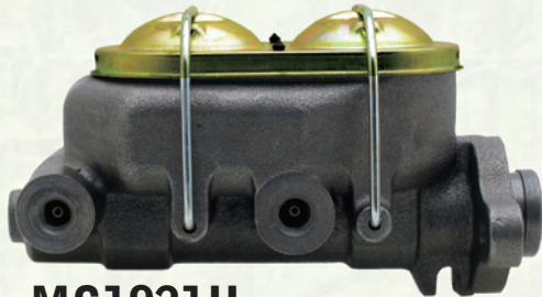
MC1921H 1" Bore. 9/16" and 1/2" ports on left side
